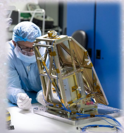
MSolo on vibration test fixture
